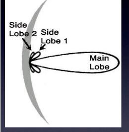
Separation and width of sidelobes is exaggerated for visibility. Sidelobe 1, for instance, is only 0.2° wide.
