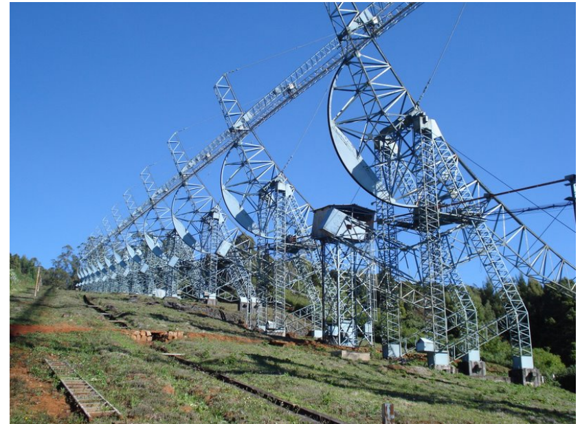
The Ootacamund (Ooty), India off-axis parabolic cylinder 530 m long and 30 m wide (15,900 m 2 ) operating at a nominal frequency of 326.5 MHz.
