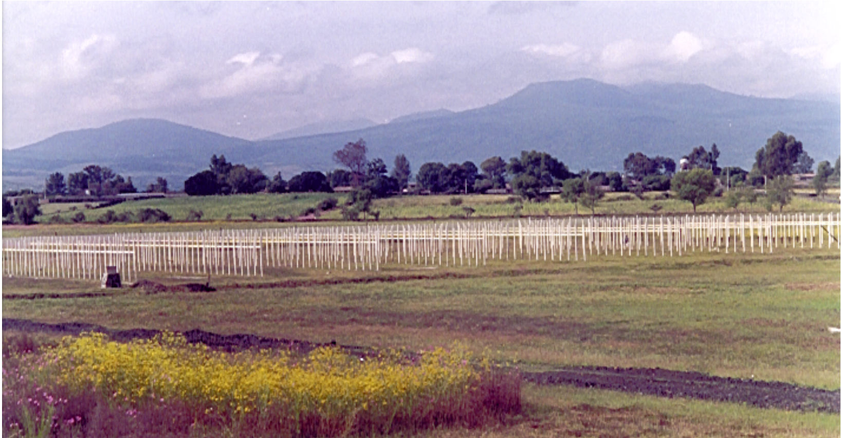
MEXART IPS 9,600 m 2 140 MHz IPS radio array near Michoacan, Mexico
