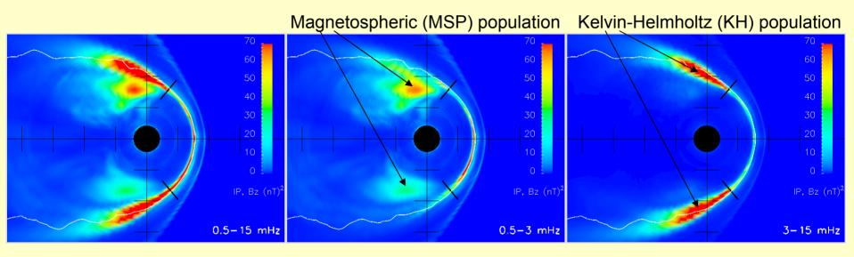
Equatorial plane cuts of  $B_z$  integrated ULF wave power from the 800 km/s simulation, integrated over three different frequency bands: 0.5–15 mHz (left), 0.5–3 mHz (middle), 3–15 mHz (right). The black ticks perpendicular to the magnetopause mark the point along the boundary where the KH waves are generated.
