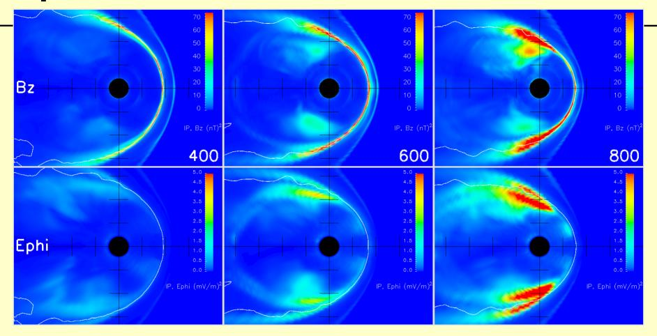
Equatorial plane cuts of ULF wave power, integrated from 0.5 to 15 mHz for the simulation  $B_z$  (top row) and  $E_{\varphi}$  (bottom row) for the three simulations in this study (columns). The white contours represent the approximate location of the magnetopause. Color scales are the same in each row to emphasize the increasing intensity of ULE wave power as the solar wind speed is increased.
