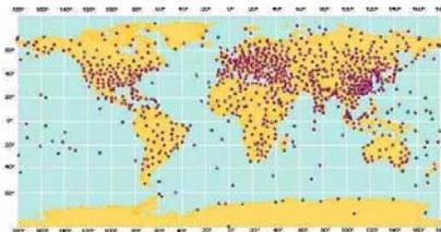
From a network of roughly 900 upper-air stations, radiosondes, attached to free-rising balloons, make measurements of pressure, wind velocity, temperature and humidity from just above ground to heights of up to 30km
