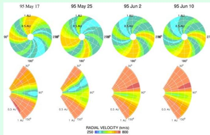
Ecliptic (top) & meridional (bottom) slices through 3D MHD numerical simulation volume for CR1896.
