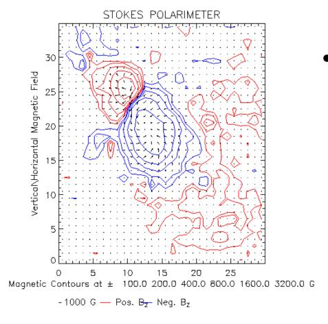
Can measure vertical (contours) and horizontal (arrows) components of magnetic field in the photosphere
