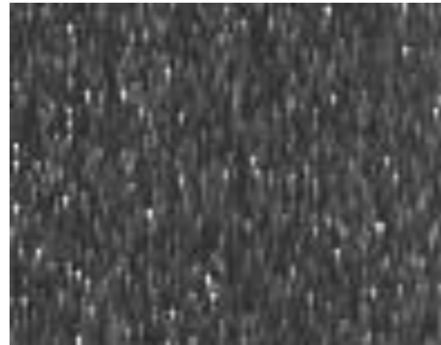
Dark Spikes and CTI damage - 1.8 \times 10^{10} 10 MeV protons/cm 2
